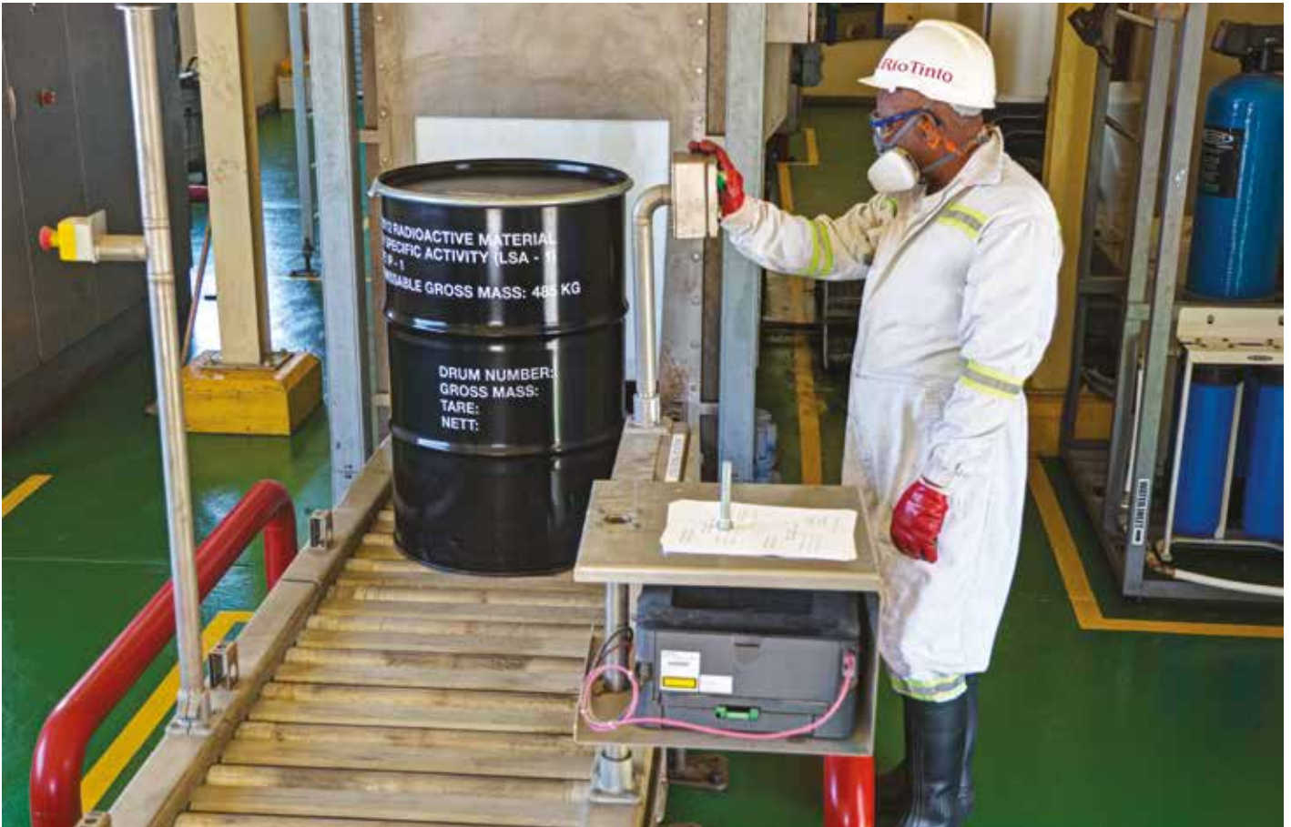
Operator Immanuel Witbooi, checking a drum filled with uranium oxide at the new automated drumming facility at the mine's Final Product Recovery operation.
