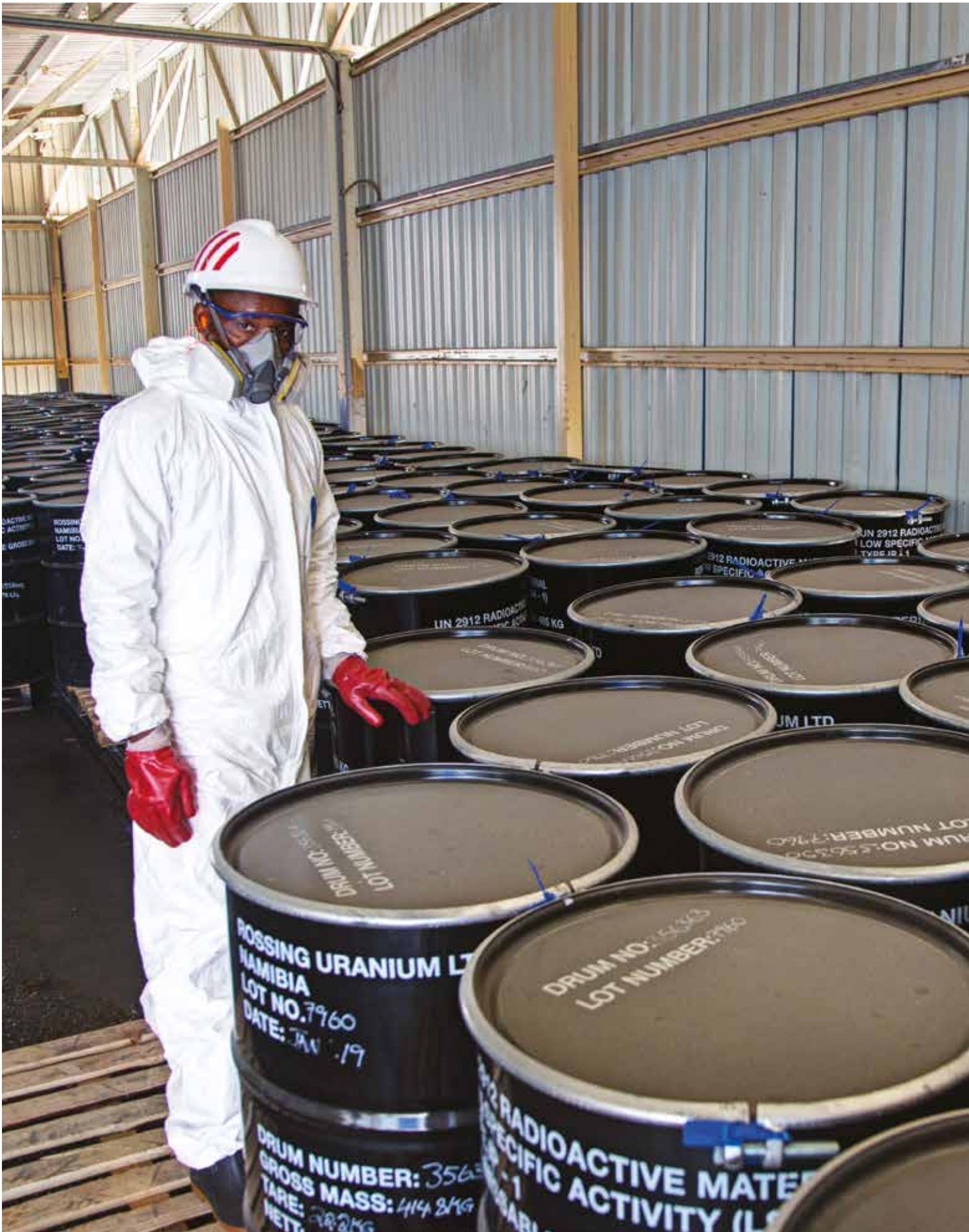
The Final Product Recovery section at Rössing Uranium is responsible for the extraction of uranium from ore mined and processed through a number of stages to produce uranium oxide ( U_3O_8 ). Securely drummed and packed, the uranium is shipped to our customers for further conversion. We produced 2,479 tonnes of uranium oxide in 2018.
